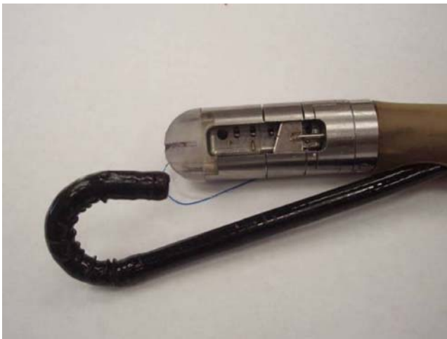
Figure 2 5 cm long rigid distal excision and suture capsule with transnasal endoscope in a retroflexed position. The guillotine excision blade is half way advanced and visible within the excision trough.
