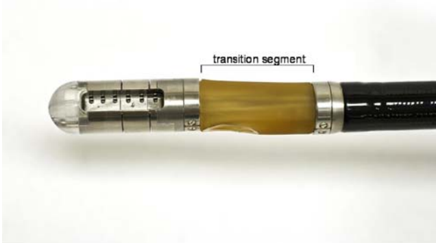
Figure 3 Capsule with flexible transition that allows introduction through the oro- and hypopharynx.
