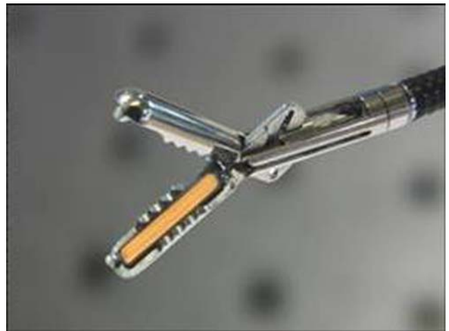
Figure 5 Prototype bipolar coagulation tool (Ethicon Endosurgical, Blue Ash, OH) which can coapt vessels as large as 5 mm.
